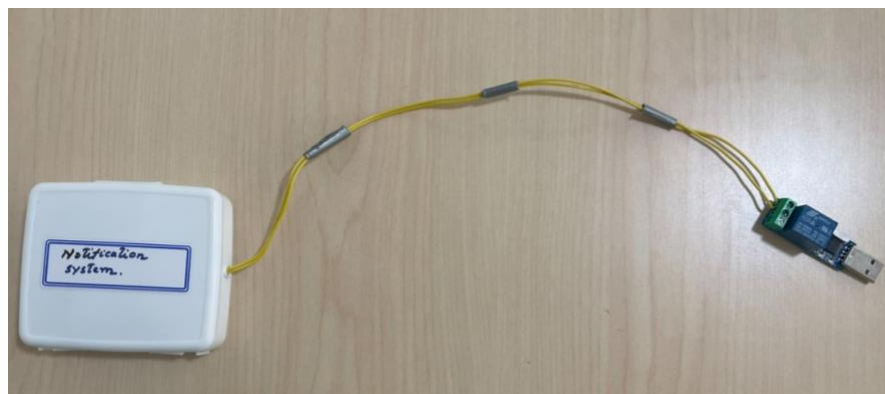
Figure 33: USB Relay and 5V Alarm Prototype
