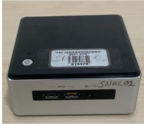
Figure 34: Intel NUC - NUC5i3RYH MiniComputer
