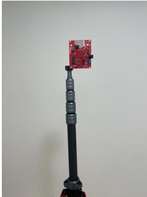
Figure 27: mmWave Radar IWR1443BOOST used for the Final Design
