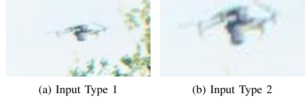
Fig. 3: Illustration of input images to the network. (a) The drone maintains its actual size in the image, but the extended bounding box may contain various background forms. (b) In the resized image, the drone no longer maintains its actual size, leading to the loss of the inherent "3D distance-bounding box size relation". Consequently, the third input form is proposed to address this limitation.
