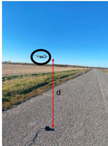
Figure 13: Experiment with the DJI mini-UAV hovering about the FMCW Radar at distance d for various experiments. This image shows the DJI mini 1.3 meters from the radar.
